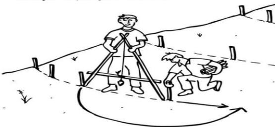
Figure 8.2: Making and using an A-frame.
